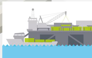
**1** The pipes are unloaded from the pipe carrier vessels and stacked on each side of the laybarge. Pipe deliveries occur regularly to maintain the 24-hour pipelay schedule.
