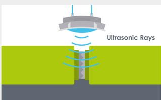
**4** The double-joint is moved to a non-destructive testing station where the weld undergoes testing to detect any unacceptable flaws. If required, the defect will be removed and the weld re-tested to ensure it meets international standards.
