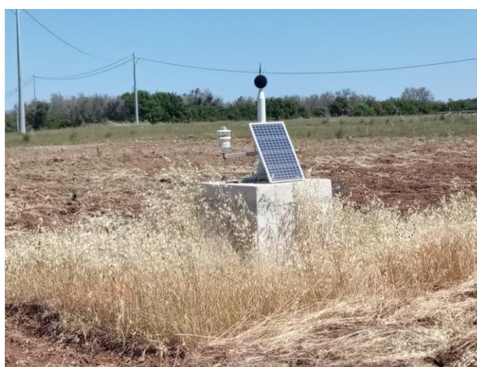
Figure 6.39: Noise monitoring station
